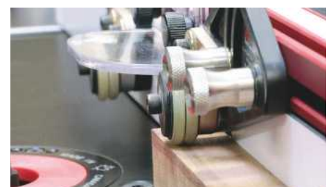
▲ The wheels toe in to pull the stock tight to the fence as it progresses
